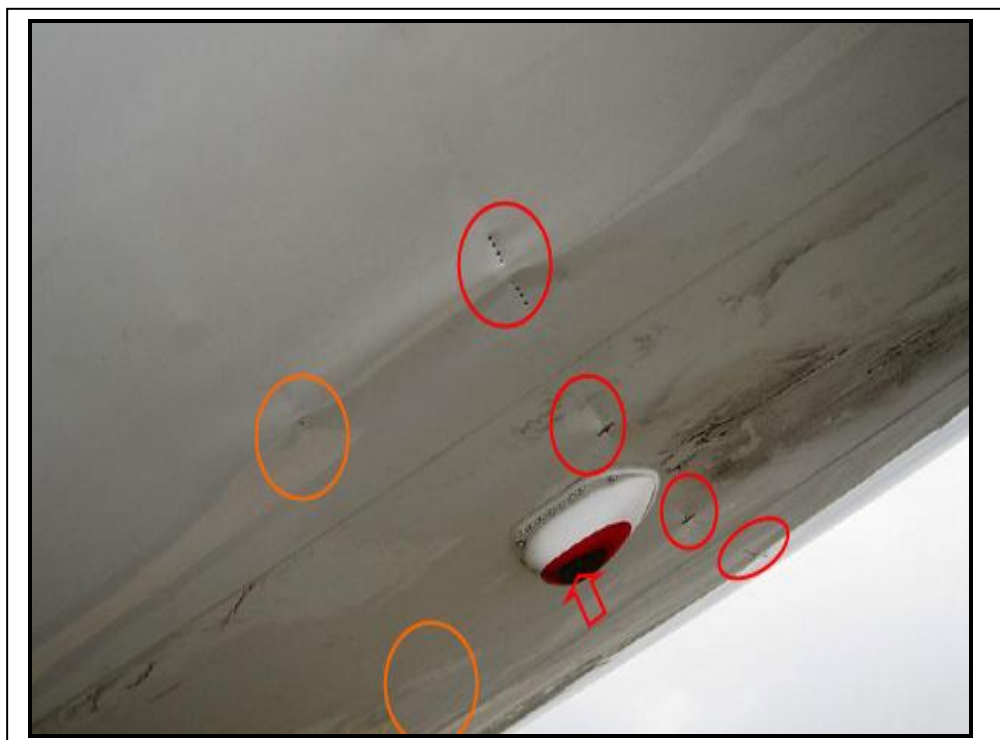
Photo nº2: View of tail skid shoe and surrounding area damage
