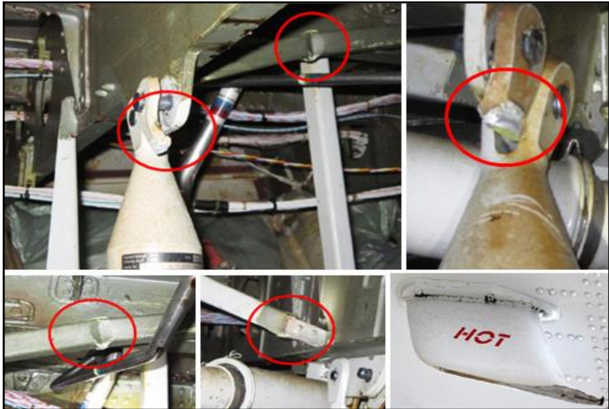
Photo n°4: Tail internal structure damage
