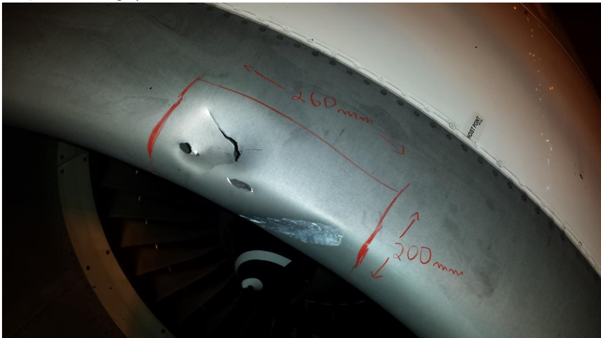
Figura 1 - Duas amolgadelas (260mm x 200mm) com um rasgo profundo || Figure 1 - Two dents (260mm x 200mm) with a deep groove
