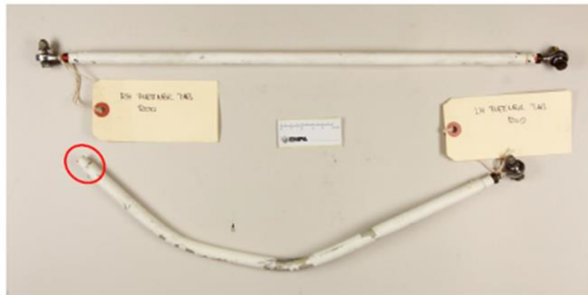
Figure 15: LH and RH elevator Flettner-tab as removed from A/C
