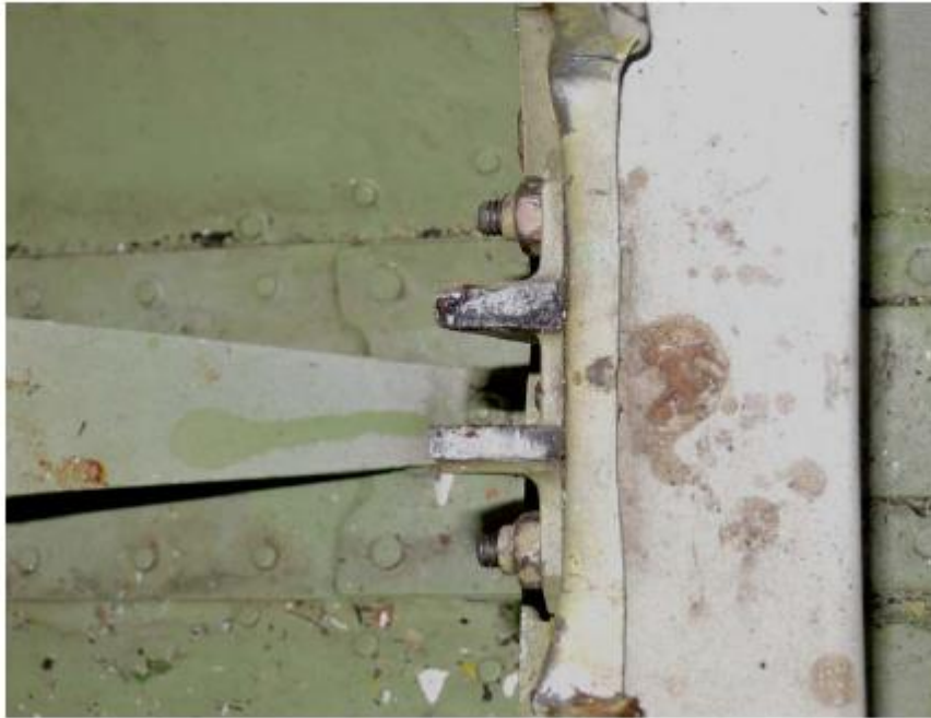
Figure 12: HT-trim attachment in unchanged condition with black contamination on the fracture
