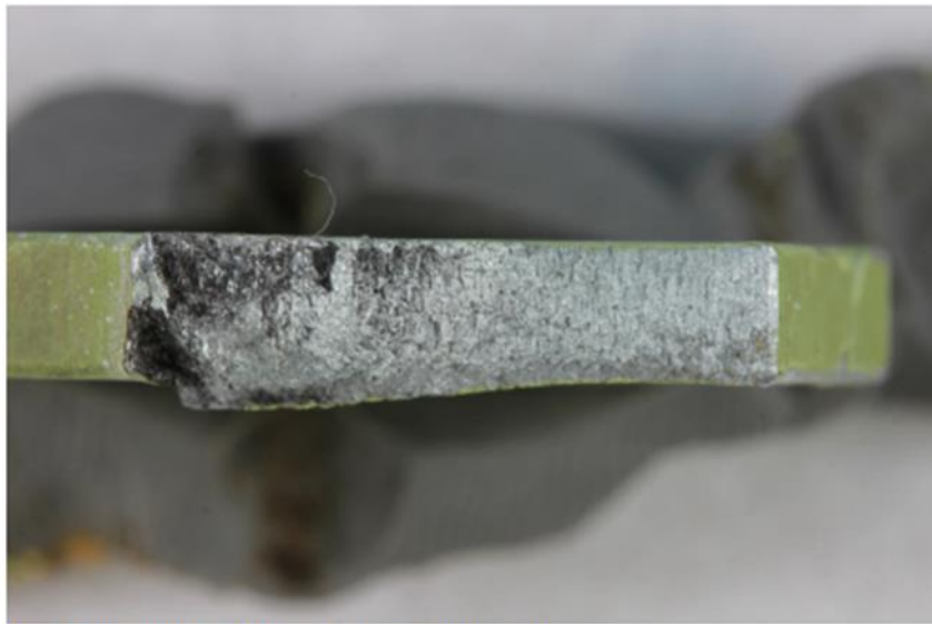
Figure 4: Overview of the LH fracture (actuator side fragment)
