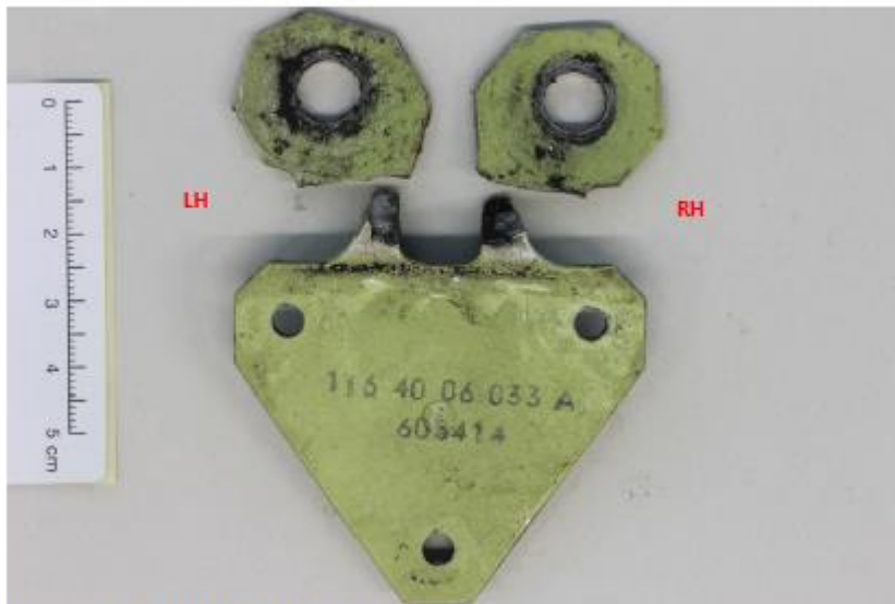
Figure 2: Overview of the failed fitting with P/N
