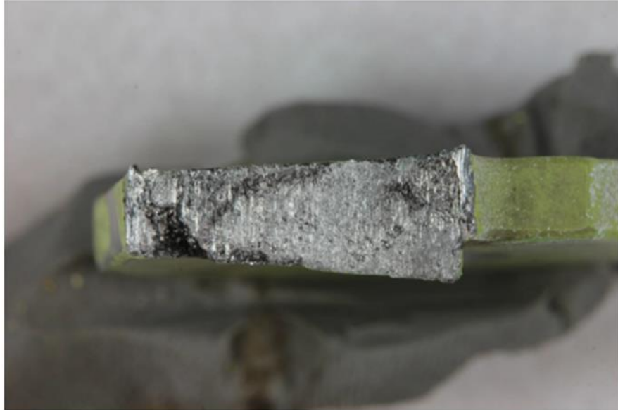
Figure 3: Overview of the RH fracture (actuator side fragment)
