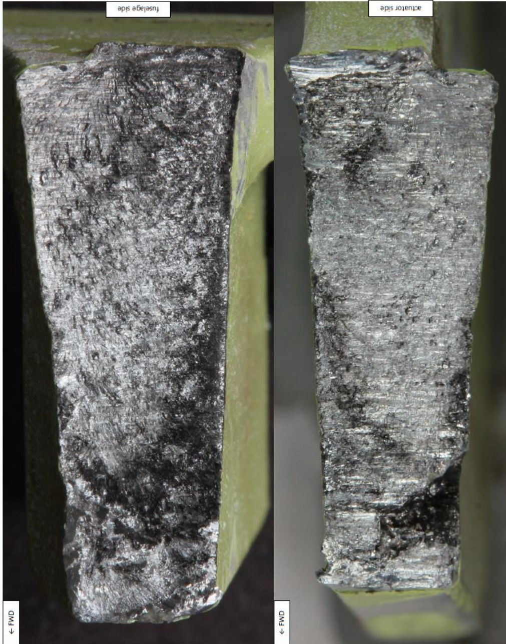
Figure 14: Condition of the cleaned fuselage and actuator side RH fracture surfaces in cleaned condition
