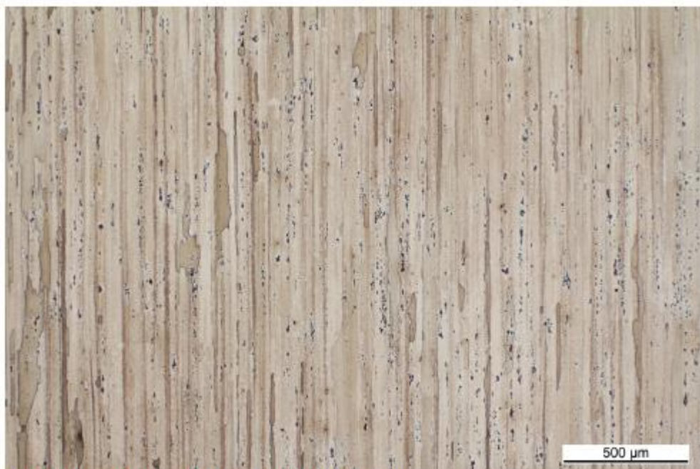
Figure 8: Etched microsection in <L> direction (section B)
